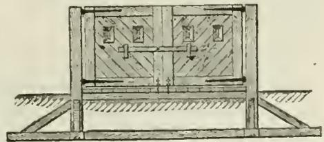
of all barriers should not be less than six feet above the ground. In the barriers with open leaves, the vertical pieces are usually extended from eighteen inches to two feet above the top rails, and their upper ends sharpened. In those which are solid, it is usual to arrange some obstruction upon the top rail, such as sharp-pointed spikes, broken glass, etc., to interfere with persons climbing over the top. It is usual
