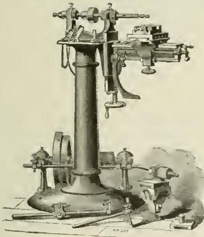
er and guide are attached is adjusted in height to suit the diameter of the cutter to be operated upon. The guide rests against the tooth that is being ground, thus gauging the work perfectly, even though there may be irregularity in the size of the teeth. The machine is adapted to cutters of all sizes and styles of teeth, whether straight, beveled, or spiral. Either small grindstones or emery-wheels may be attached to the spindle.
