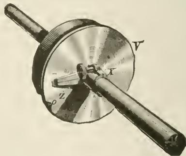
of the circle. There is a brass tomion, *V*, to fit the muzzle of the gun, with a hole through its center to receive the staff of the star-gauge. It is turned to fit snugly the bore of the piece, into which it enters two or three inches, to hold it firmly in place; and has a projecting flange or face to prevent it going in too far.
