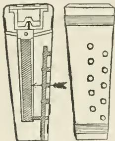
furnished on the inside with a pierced nipple for percussion-cap. The upper edge of the hollow cylinder is flanged in such a manner as to rest on the top of the stock; thereby preventing the igniter from being driven bodily into the fuse on discharge of the gun. Inside of this hollow cylinder the plunger is hung on a brittle wire (half copper and half
