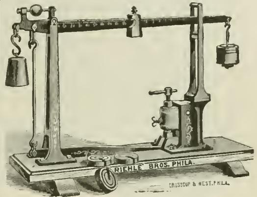
of the stand or gate. If, however, it should not, the beam is again raised by applying pressure with the screw and moving the poise on beam until the specimen breaks or the desired test is applied. See *Testing-machine*.
