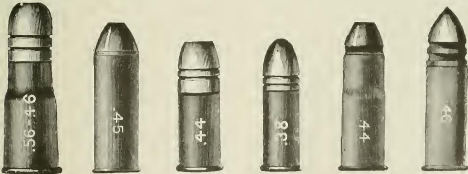
Central-fire Solid-head Reloading Cartridges.—Pistol.
