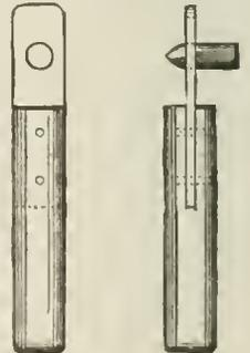
be removed from two or three hundred before working at the powder. A small brass pick and scraper combined is used, with the edges and point sharpened, with which the wad is removed and the interior of the shell scraped.
