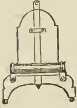
This instrument is frequently called the *gunner's perpendicular*.
