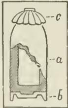
inches. A corrugated cap of tinned sheet-iron, *c*, is used with 3-inch projectiles to catch and direct that portion of the flame of the charge which escapes over the projectile on to the fuse to ignite it. See *Expanding Projectiles*.
