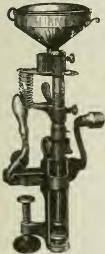
This machine loads very quickly, and during the operation of loading the cartridges the powder is inclosed in a covered reservoir. The cartridges are loaded uniformly, and the wads squarely placed, thus improving the shooting of the gun. An adjustable shelf adapts the cartridge-receiver to loading shells of any length. The machine can be carried in a gun-case, occupying smaller space than the paraphernalia in general use. No practice is
