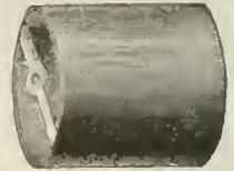
**CYLINDER-MILL.**—One form of a mill for pulverizing the ingredients of gunpowder, having a cylindrical runner traversing on a bed-stone. See *Gunpowder*.
