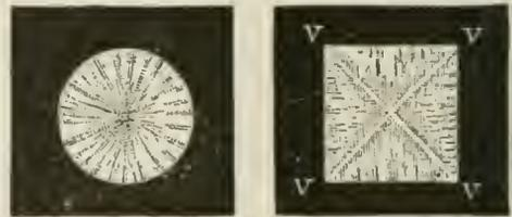
radiate from the center; in the square bar they are arranged perpendicularly to the four sides, and hence have four lines in the diagonals of the square—in which the terminal planes of the crystals abut or interlock, and about which the crystallization is always confused and irregular. The result of this arrangement is to create *planes of weakness* where the different systems of crystals intersect.
