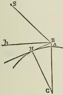
A be a point on the surface of the earth, and B a point situated in a vertical line from A. Let BH be a tangent to the earth's surface drawn from B, B*h* a line in the same vertical plane perpendicular to AB. The angle *hBH* is the *true dip* of the horizon to a spectator at B. The true dip measured in minutes is equal to the distance in nautical miles of the visible horizon. Let C be the center of curvature of the surface; then, since CHB
