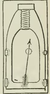
**FRENCH SIGHTS.**—In this system, employed when the target is invisible, specially constructed sights (used in the ordinary sight-slots) are provided, having cross-bars on their heads, divided into scales of equal parts, and parallel to the axis of the trunnions.
