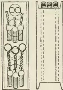
To pack the primers, rectangular wooden blocks are made, having holes .38 inch and .57 inch in diameter, bored in two opposite ends. The primers are placed in the holes, 5 or 10 to each block. The block is covered with a paper wrapper, which is then varnished. A printed label tells contents, place, and year of manufacture. The blocks are packed in wooden boxes containing 1000 of five primers each, or 100 of ten each. For
