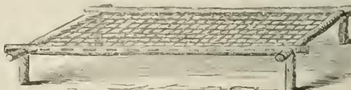
ants are numerous. A very comfortable bed, shown in the drawing, is made on the principle of a tennis-player's racket; being a framework of wood, with strips of raw-hide lashed across it from side to side and from end to end. It is the *Angareb* of Upper Egypt, and may be readily constructed in the field. See *Camp-bedstead*.
