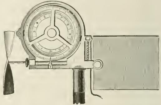
shows this instrument adapted for use in small rivers and streams, or to show the number of gallons flowing from any reservoir or vessel. The mean velocity
