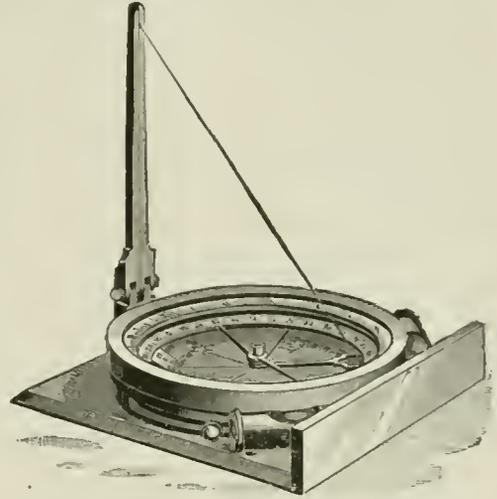
is made equal to that of the latitude required. In using the dial-compass it is first leveled carefully, the equation of time for the given day allowed for, and then by observation on the sun at midday the true meridian approximately obtained. The needle may then be set to the meridian by laying off the variation, and any deflection of the needle from the true meridian will indicate the presence of veins of magnetic iron-ore. See *Clinometer and Solar Compass*.
