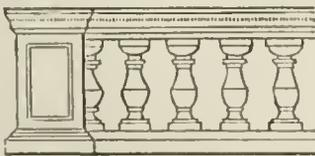
The balustrade is often used as a parapet over bridges, for the roofs of large edifices, etc., or as a mere termination to the structure. It is also used to inclose stairs, altars, balconies, etc. Balustrades are made of stone, metal, or wood. See *Fortification*.
